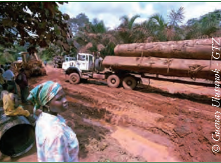
Photo 4.2: Regular use by logging trucks can damage rural roads.
