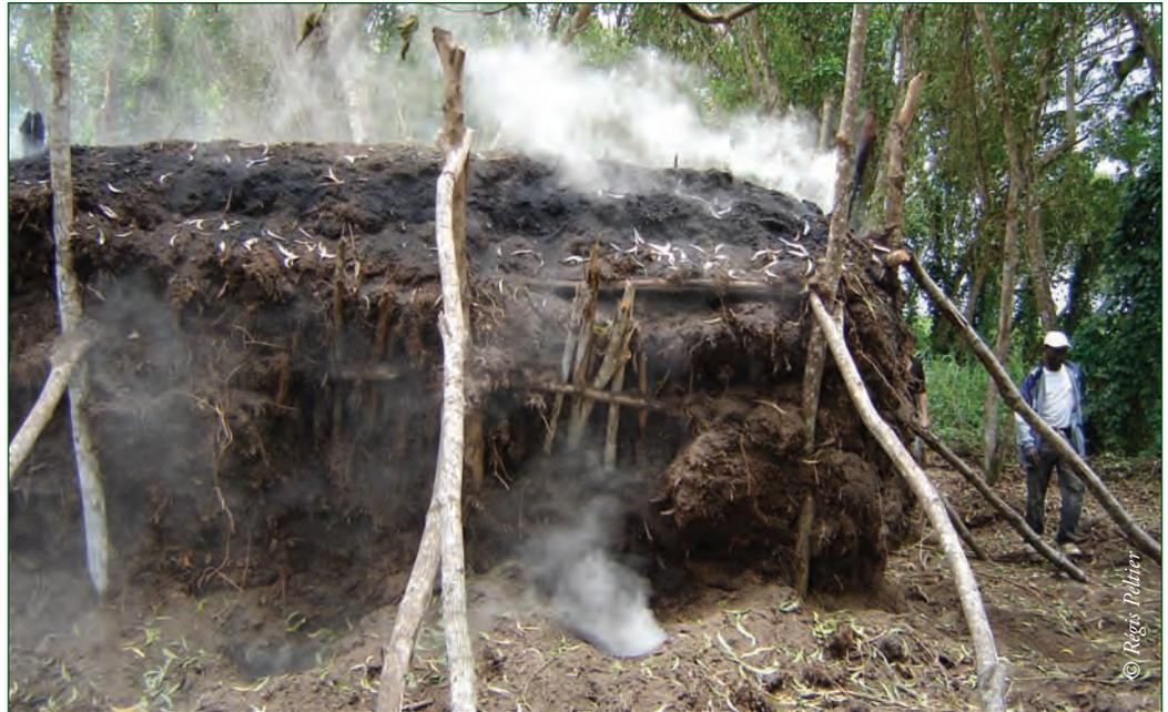
*Photo 13.5: A charcoal furnace, which can operate for several weeks at a time.*
