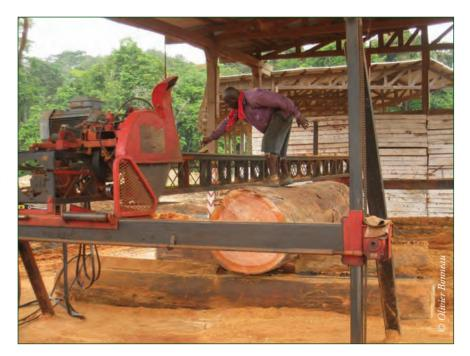
Photo 12.7: The mobile saw "Mighty Might" is used to cut logs on site (Gabon).
