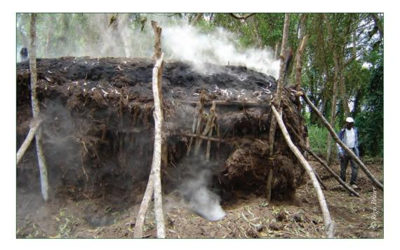
Photo 13.5: A charcoal furnace, which can operate for several weeks at a time.
