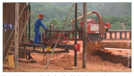
Photo 16.6: Sawing on site reduces the volume of wood that has to be transported.
