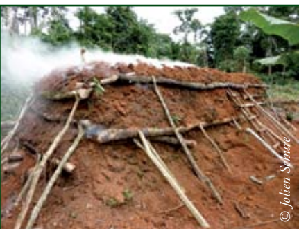
Photo 5.3: Charcoal production oven, Cameroon
