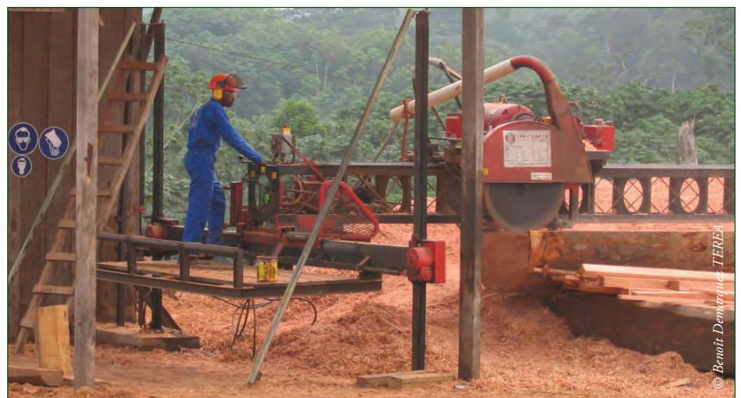
*Photo 16.6: Sawing on site reduces the volume of wood that has to be transported.*
